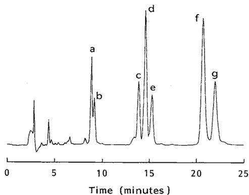
Column conditions: Column; Cosmosil-AR 4.6 i.d. × 250 mm, solvent; acetonitrile-0.5% triethylammonium phosphate buffer pH 3.0 (45:55), flow rate; 1.0 ml/minute, detector; UV (230 nm).
